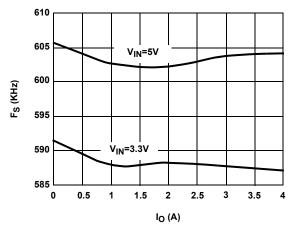
FIGURE 7. F<sub>S</sub> vs I<sub>O</sub>
