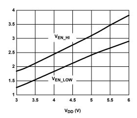
FIGURE 5.  $V_{EN\_HI} \& V_{EN\_LOW} vs V_{DD}$
