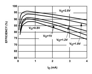
FIGURE 2. EFFICIENCY ( $V_{IN} = 3.3V$ )
