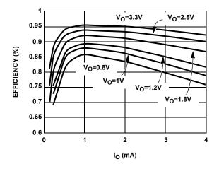
FIGURE 1. EFFICIENCY ( $V_{IN} = 5V$ )
